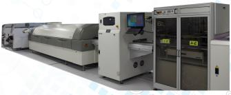
The solution provided, consists of an in-line handler fitted with a vision system. The camera software is capable of learning the position of all LED's on a new pcb, thereby reducing the time to introduce a new product. In addition to identifying the location of any missing or faulty LED's the tester measures the colour temperature of every pcb. An image is taken of faulty units with the location of any missing LED's identified.
